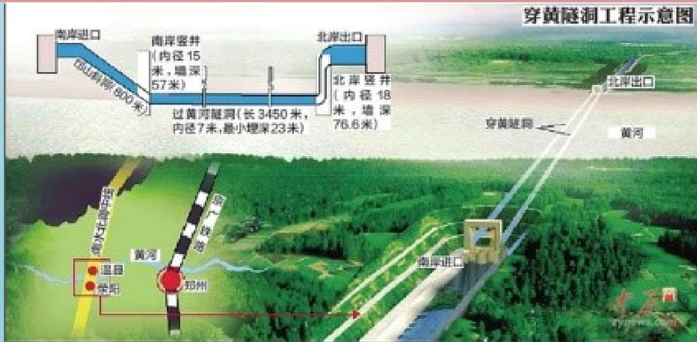
Pass under Yellow River , length 4250m, discharge  $500\text{m}^3/\text{s}$ , tunnel diameter  $2 \times 7\text{m}$ .
